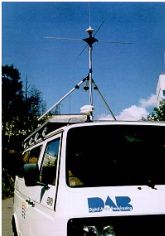
Figure 3 ▲ DAB measurement van with vertical and horizontally-polarized antennas on the ground plane.
