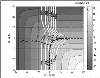
Figure 5: Achievable rates 0.25...1.75 bit/s/Hz for a two-Tx system with an applied random phase and optimal detection
