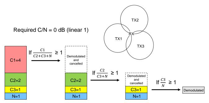
Figure 3: Example of SIC; the weakest Tx3 signal (received with power C3) is demodulated in three steps
