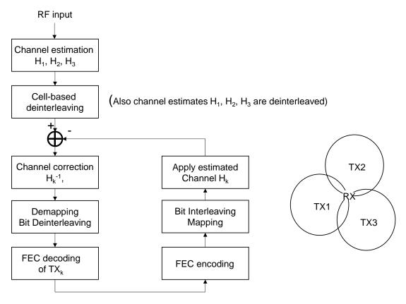
Figure 7: Simplified diagram of receiver processing of channel estimation and interference cancellation
