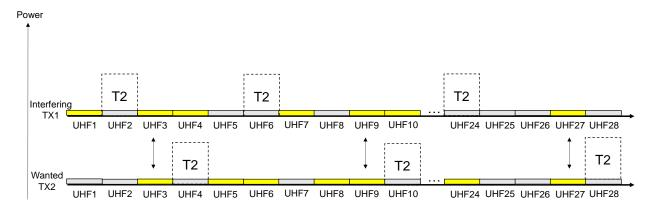
Figure 8: WiB interleaved with DTT
