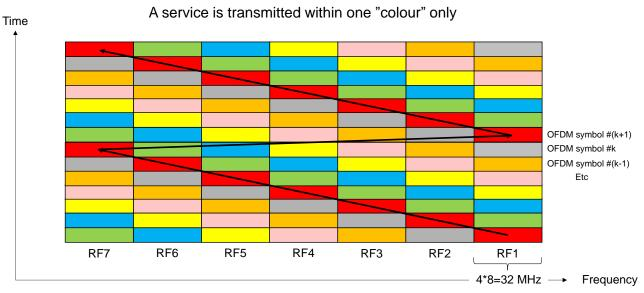
Figure 2: A possible TFS transmission scheme
