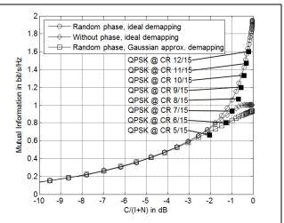
Figure 6: For C/I=0 dB, achievable rates for various de-mappers. Included is the performance with ATSC 3.0 CRs (■)
