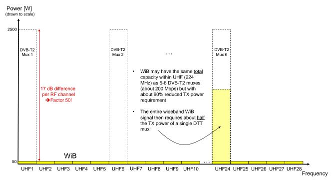
Figure 1: Required power for DVB T2 and WiB
